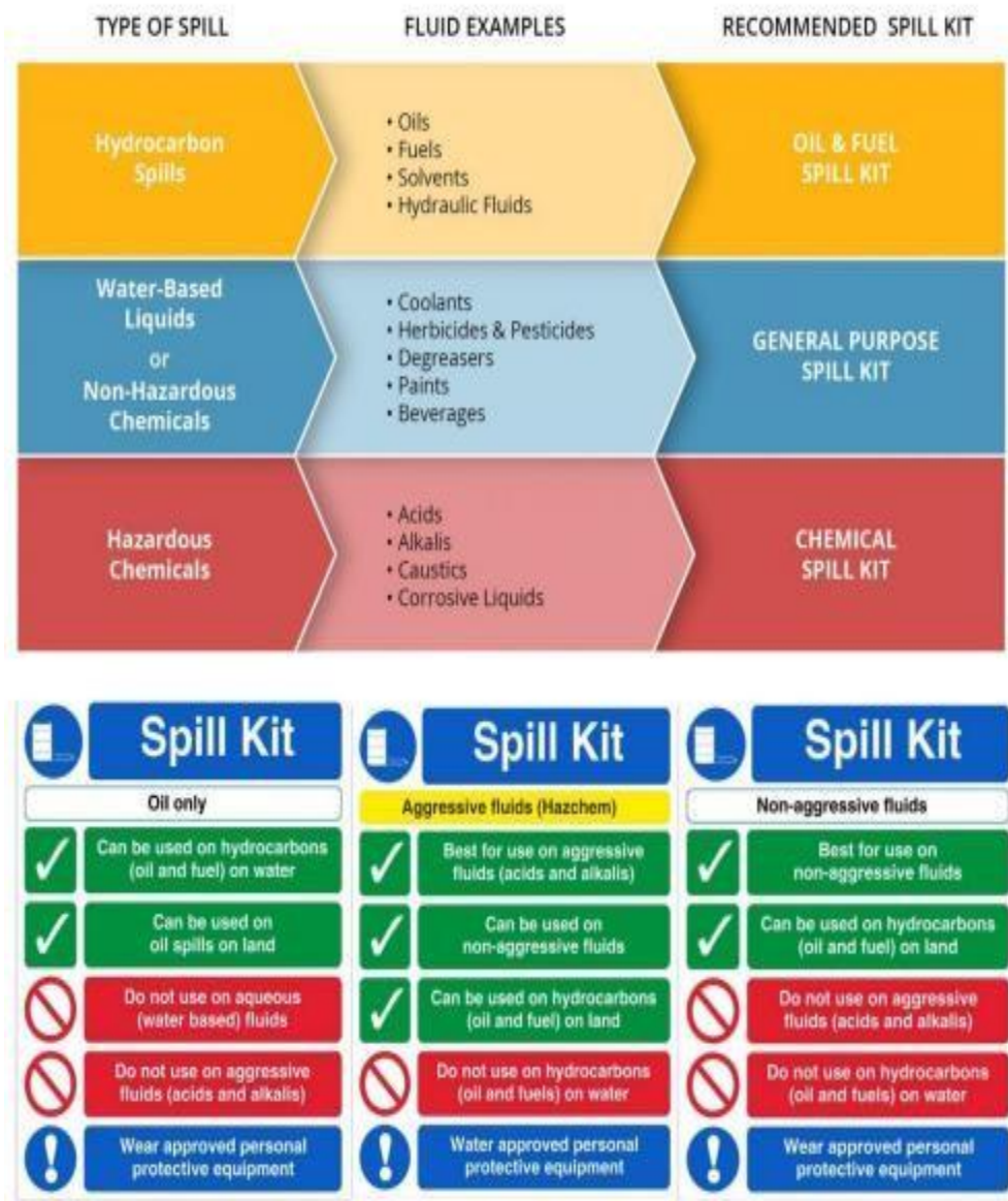
Figure 7-12. Examples of signs to be installed near spill kits on site
