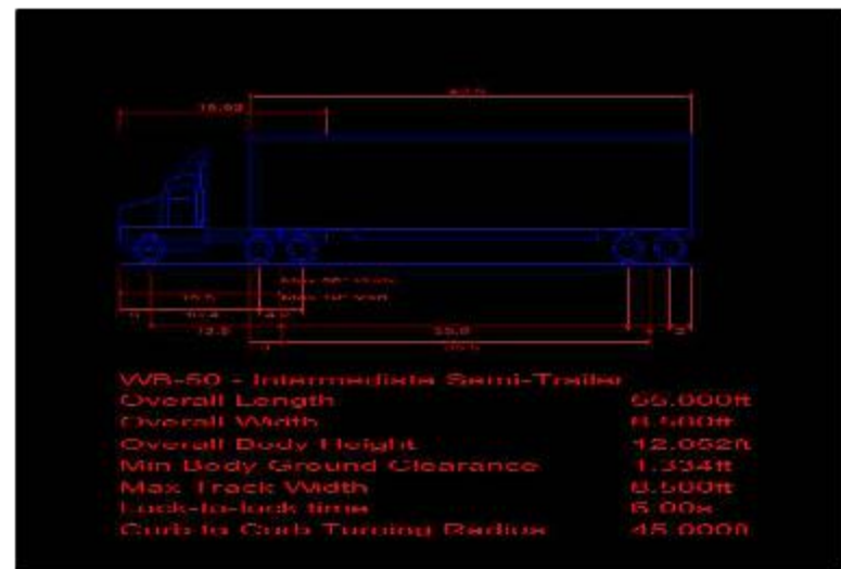
WB-50 SEMI-TRAILER DIAGRAM
